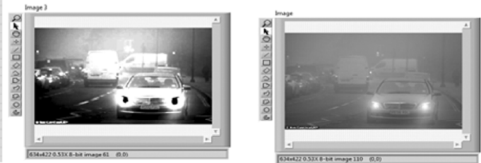
Figure 6: Output for the modified Image Processing Algorithm by using the Median Filter
