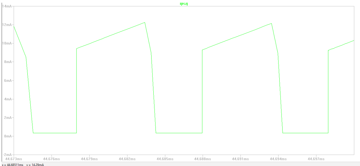
Figure 3: Current sensed through the inductor
