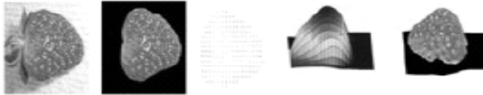
Figure 4: Shape from texture (From left to right: Original image, Segmented texture region; Surface normal; Depth map; Reconstructed 3D shape) (Fig reference 15)
