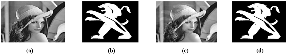
Figure 3: (a) Original image (b) Watermark Image (c) Watermarked image (d) Recovered Watermark Image
