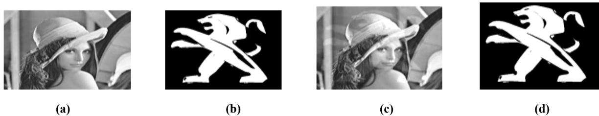
Figure 5: (a) Original image (b) Watermark Image (c) Watermarked image (d) Recovered watermark Image
