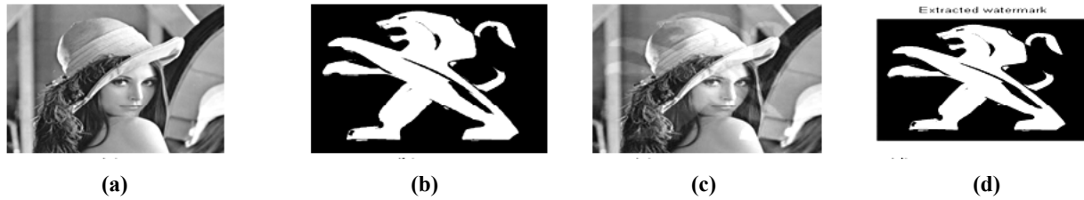
Figure 1: (a) Original image (b) Watermark image (c) Watermarked image (d) Recovered Watermark image
