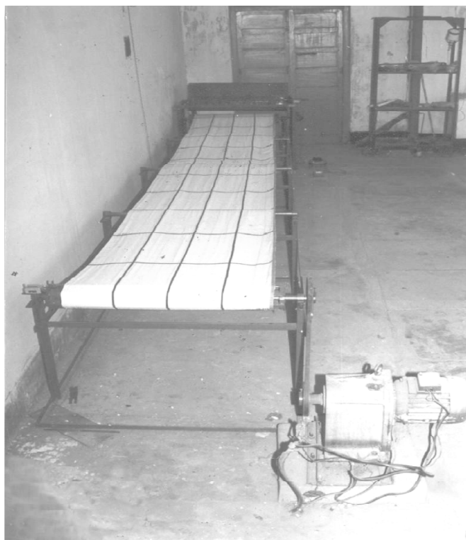
Figure 1: Test Rig for Metering of Seeds through Sticky Belt
