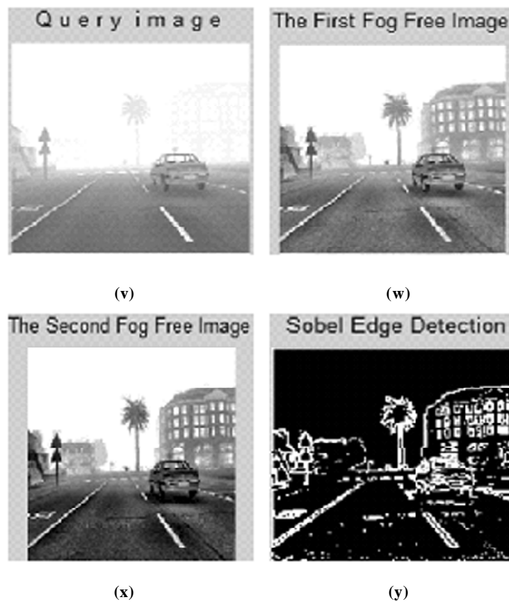
Figure 6: (v) Original Fog Image (w) Our Proposed Result of First Fog Free Image (x) Our Proposed of Second Fog Free Image y) Edge Detected Image
