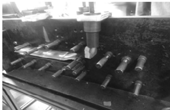
Figure 11: Before pin modification the pins are not properly linked with required part
