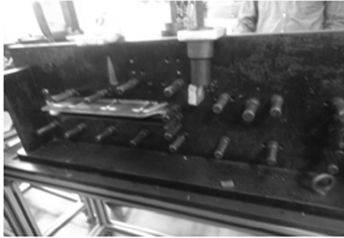
Figure 12: After pin modification the pins are properly linked with required part
