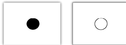
Figure 10: Threshold image before and after edge detection with a 2D Sober convolution filter
