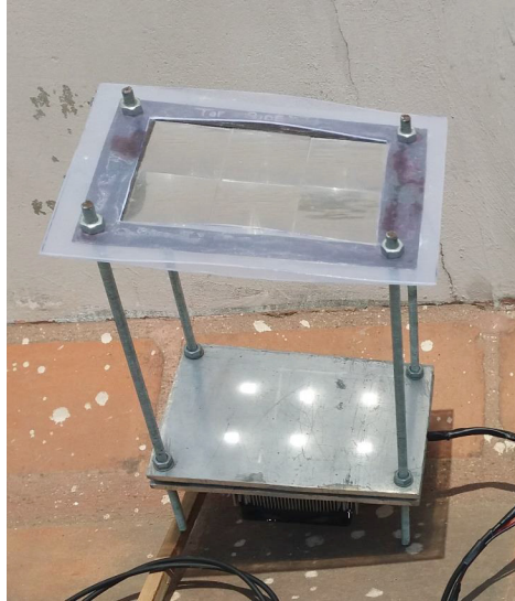
Figure 6: Series connected TEG Modules with Fresnel lens setup
