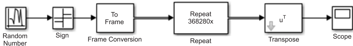
Figure 5: Simulink model for generating data components for E1-B
