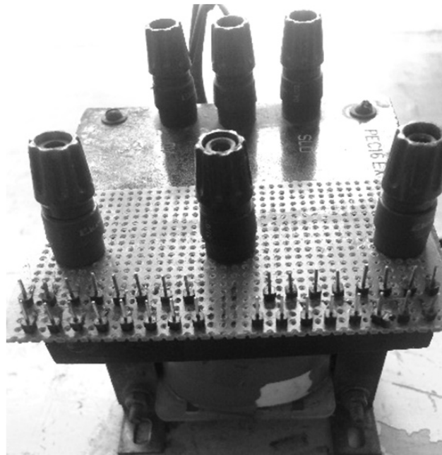
Figure 9. Practically designed transformer 230/24v
