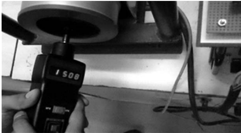
Figure 10: Speed of the BLDC motor at 1508 rpm
