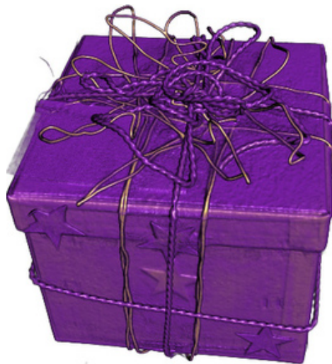
Figure 3: Present: An industrial CT scan of a Christmas present
