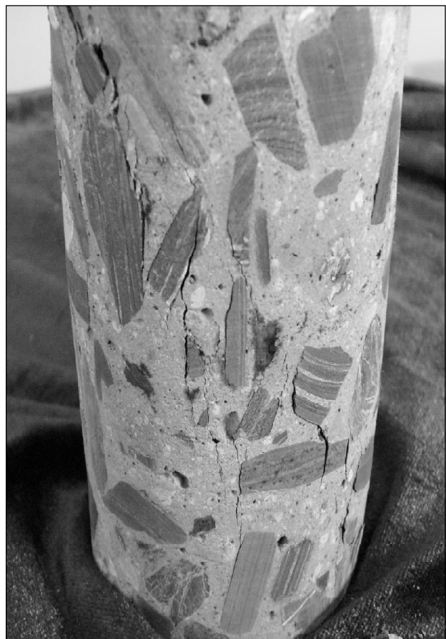
Figure 4: Failure Mode of PMFRCC in Compression
