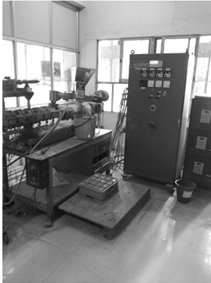
Figure 3: Twin Screw extruder–process of hybrid fiber bio composite preparation
