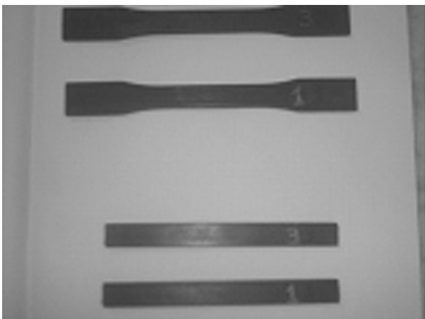
Figure 4: Tensile, flexural and impact test specimens of PBA/Si composites.
