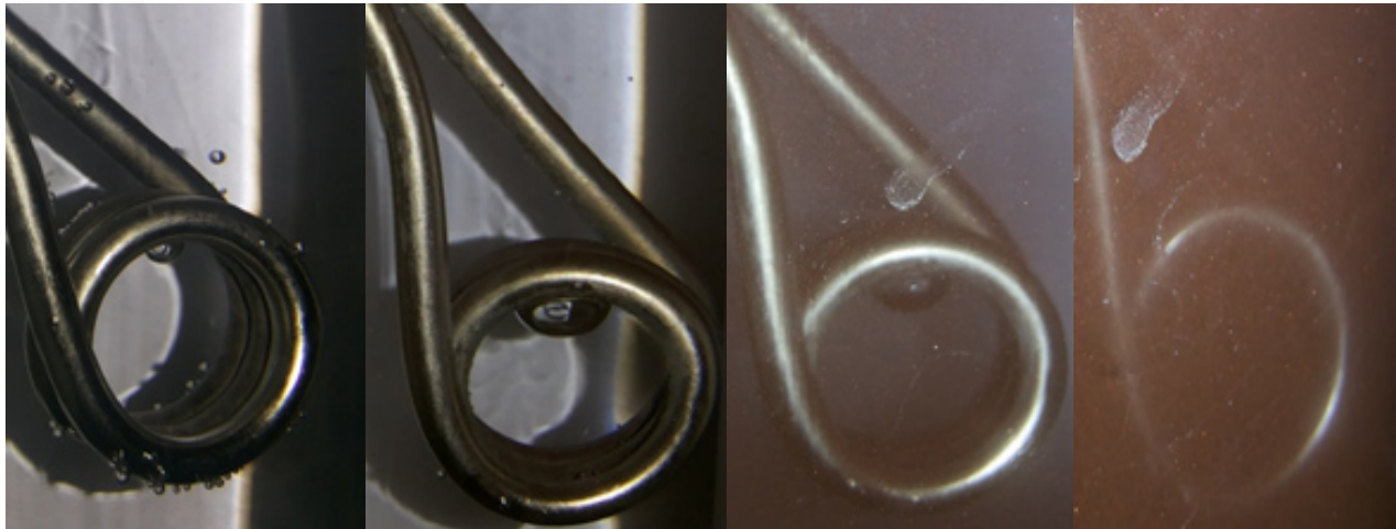
Figure 3: These images at 140 Volts at 70°C of Pure water, 80 ppm of copper, 400 ppm of copper & 800 ppm of copper
