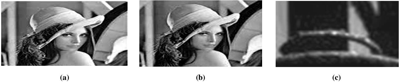
Figure 3: (a) Original image (Lena) (b) Watermarked image, PSNR = 33.72 db (c) Extracted watermark, NCC=0.8441
