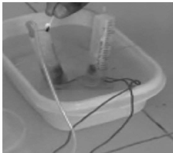
Figure 3: Generation of Oxygen through Electrolysis process
