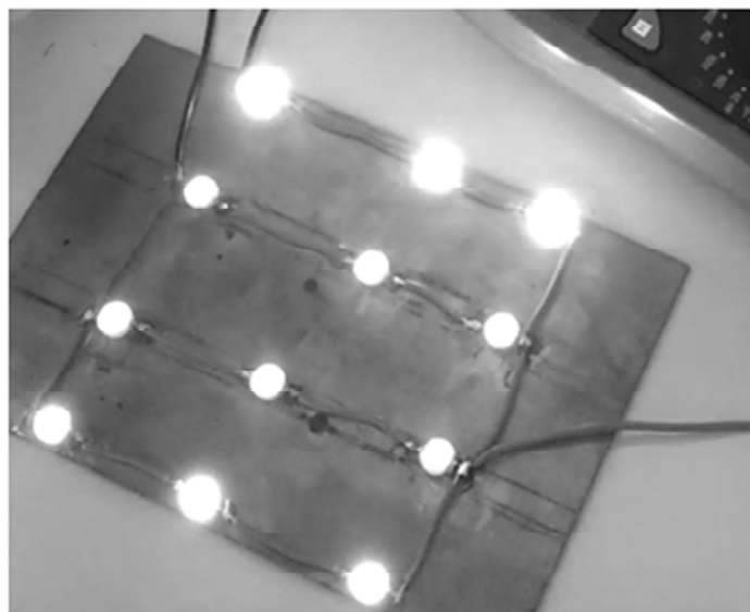
Figure 2: The fabricated LED array
