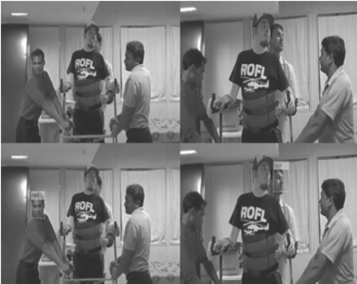
Fig. 3. Face detection using Viola-Jones Algorithm
