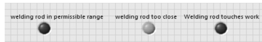
Figure 8 : Visual feedback when welding rod is close to work
