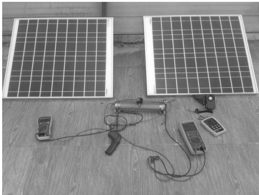
Figure 2: Experimental model of two single PV panels connected in series
