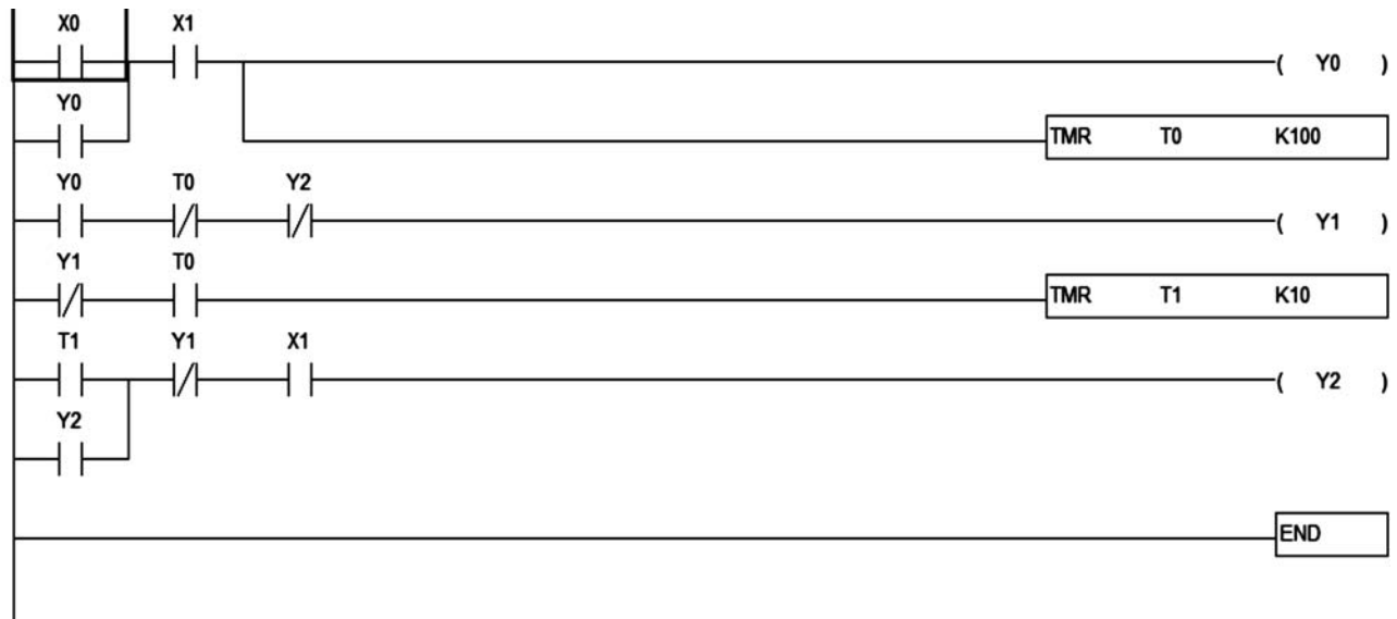
Figure 7: Star delta ladder logic program using PLC
