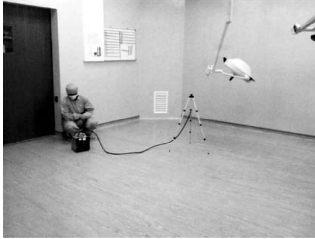
**Figure 3: PM measurement conducted in the pre-op room**
