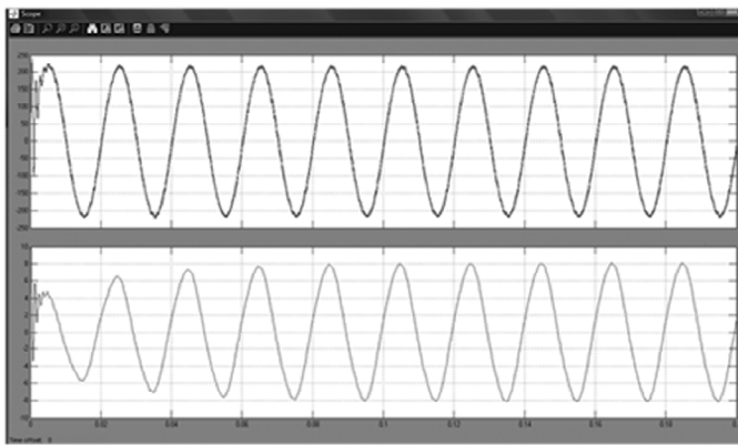
Figure 7: Source Side voltage and current waveform
