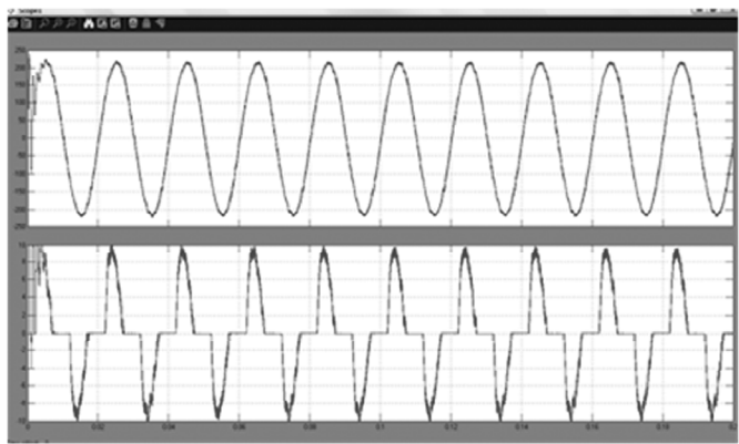
Figure 8: Load Side voltage and current waveform
