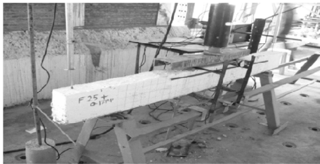
Figure 8: Flexure beam test setup
