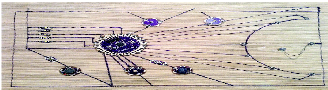
Figure 2: Lily Pad sewn to textile using conductive thread
