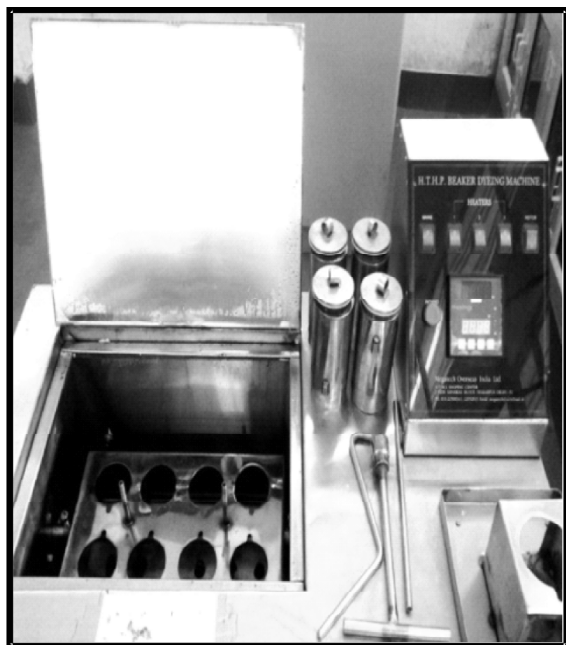
Figure 2: High Temperature High Pressure (HTHP) beaker dyeing machine
