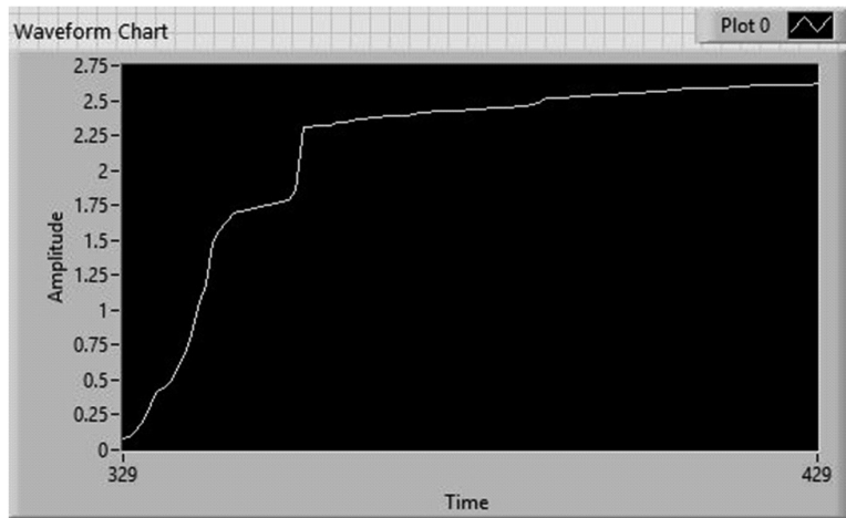
Figure 2: Step response of Fractional Order PID Controller at given values using LabVIEW
