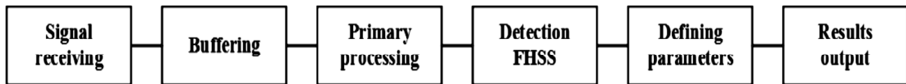
Fig. 2. Generalized diagram of the functioning of the detector for frequency hopping spread spectrum signals (FHSS).
