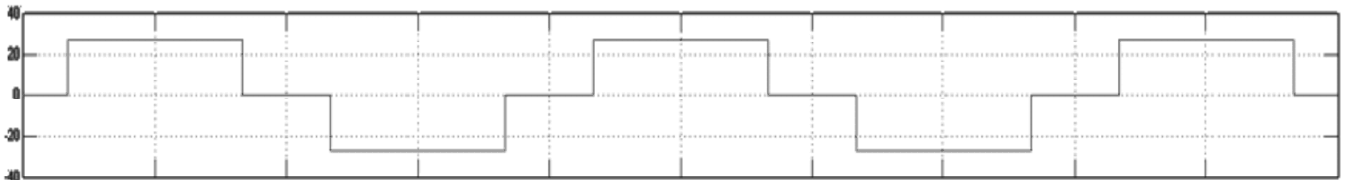
Figure 6: Output Voltage of Main Bridge in 27 level asymmetrical cascaded H-bridge multilevel inverter
