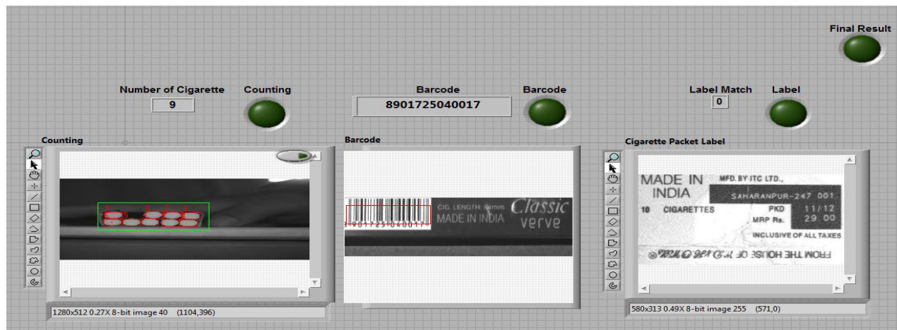
Figure 13: Off-line inspection of cigarette packets (fault in label, barcode and number of cigarettes)
