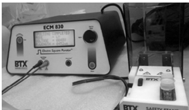
Figure 1: Electroporator ECM 830 with cuvette placed in safety stand
