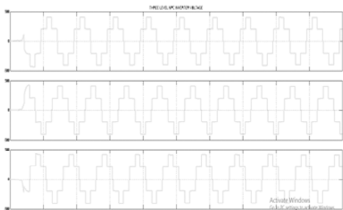
Figure 10: NPC Multilevel inverter (Three level) voltage
