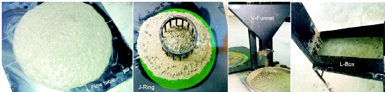
Figure 1: Workability Tests (Flow table, J-ring, V-funnel and L-Box)
