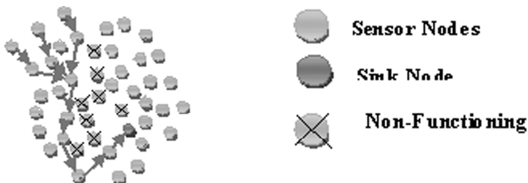
Figure 2: Routing path when some of the nodes in the network are not functioning.
