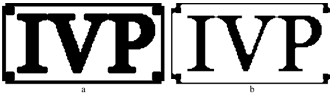
Figure 4: Opening process: the input image undergoes (a) the erosion process, which is then followed by (b) the dilation process
