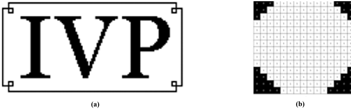
Figure 1: (a) Input image[15], (b) structuring element of a disk shape with a radius of eight pixels
