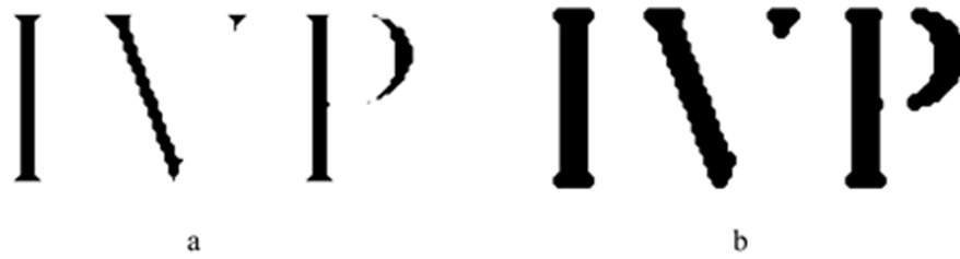
Figure 5: Closing process: the input image undergoes (a) dilation process, then followed by (b) erosion process
