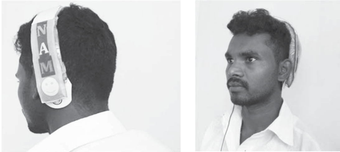
Figure 2. Self-Designed NAM microphone attached to the user
