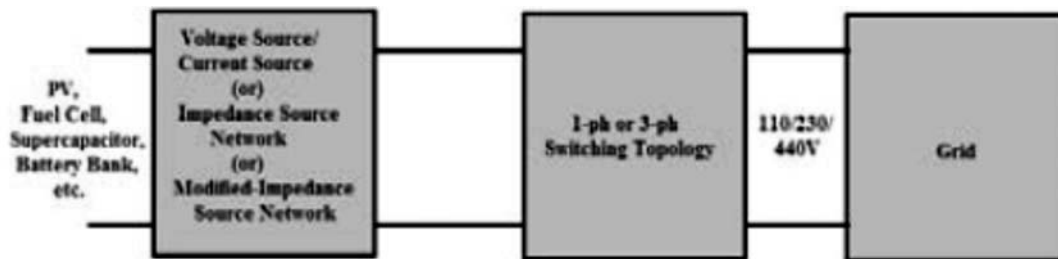
Fig. 1. Block diagram of electric power conversion between source and load.
