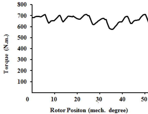
Figure 11: Torque profile of 11.1 kW RFPMBLDC motor
