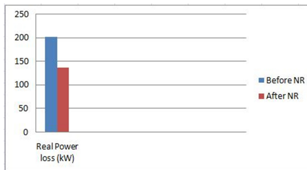
Figure 5: Comparison of Power loss before and after Network reconfiguration
