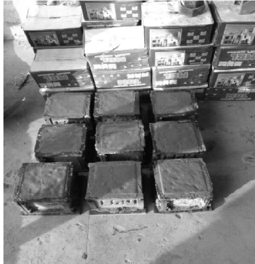
Figure 1: Casting of cubes
