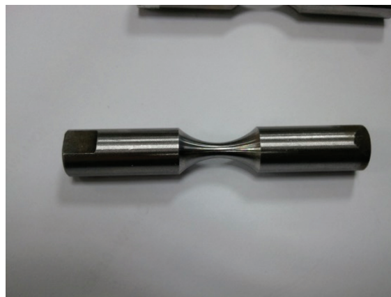
Figure 12. PMF treated Fe-34Mn-10Al-0.76C alloy specimen to be tested.
