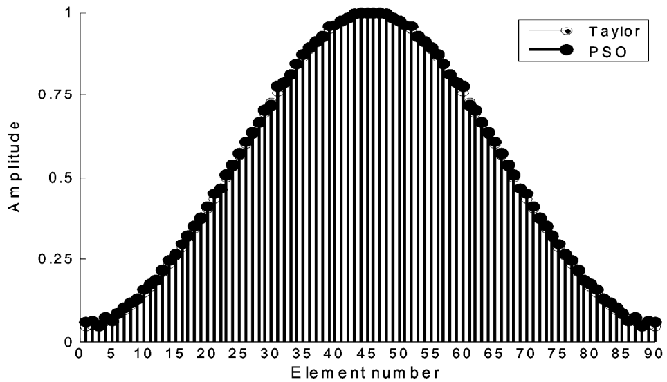
Fig. 10. Normalized Amplitude Excitations for an array of N = 90 Elements using Taylor Amplitude Distribution and PSO
