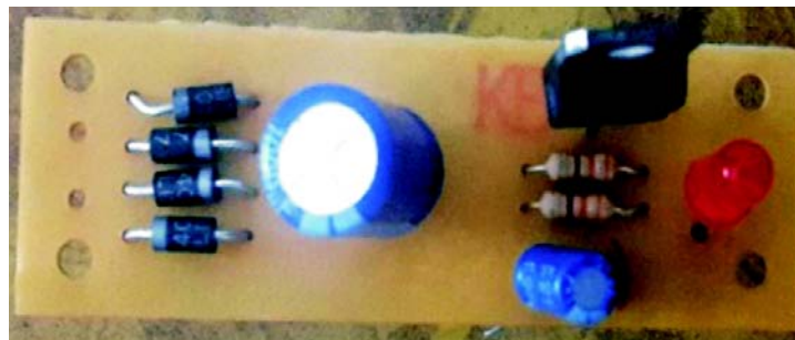
Figure 3: Power Supply Circuit on PCB
