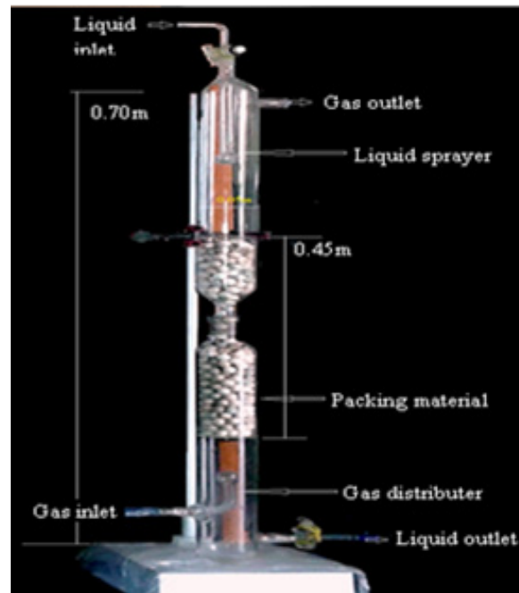
Figure 5: Photographic view of the packed column
