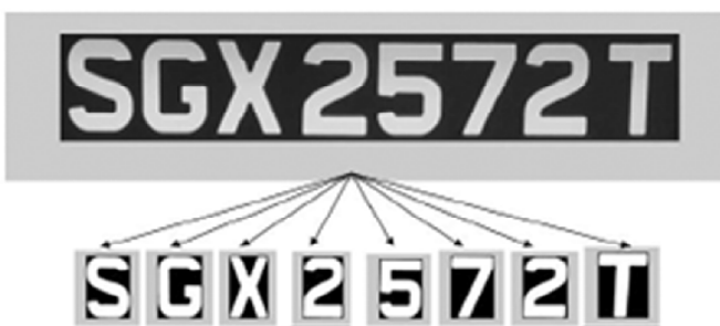
Figure 4: Segmented Number Plates and Number Extraction [2]
