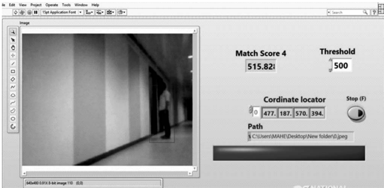
Figure 3: Template matching and person 1 detection with overlay function
