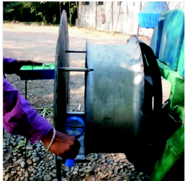
Plate 1: Measurement of blower speed and air velocity
