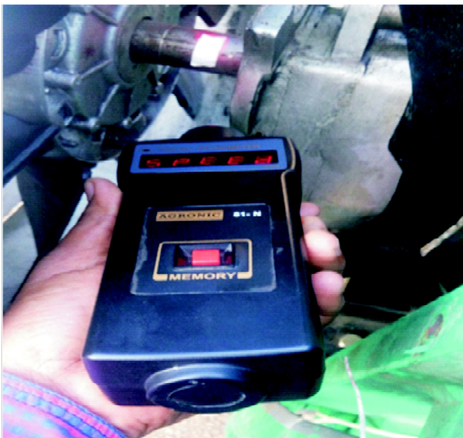
Plate 1: Measurement of blower speed and air velocity
