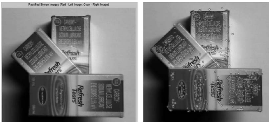
Figure 9: Rectified Stereo Image Pair and Inlier Points in the Stereo Image Pair
